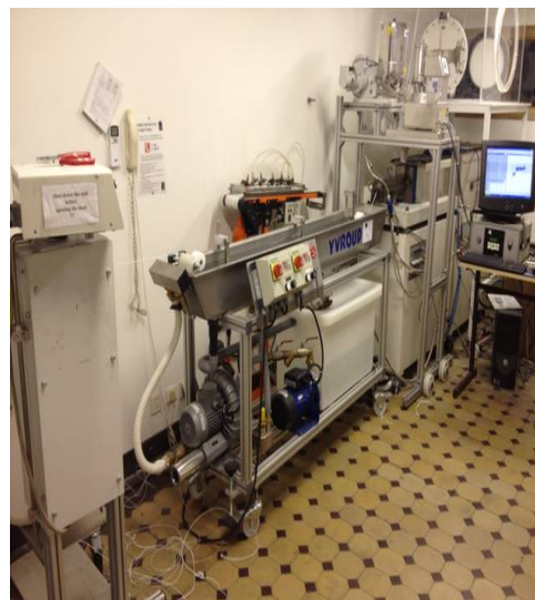
Figure 1. Compounding ( Haake Co. , England) machine for master batch for nano ZnO/PP
