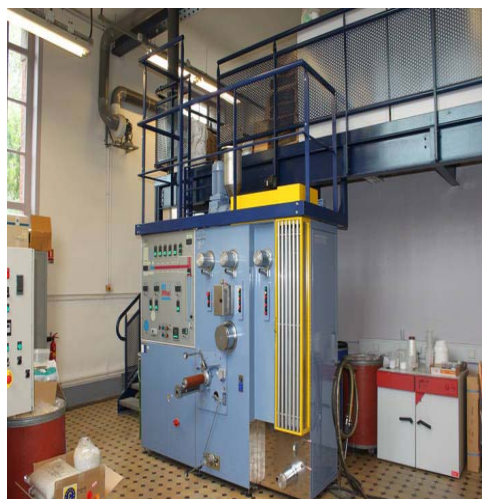
Figure 2. Extrusion and melt spinning machine (Spin Boy1) for nano ZnO/PP
