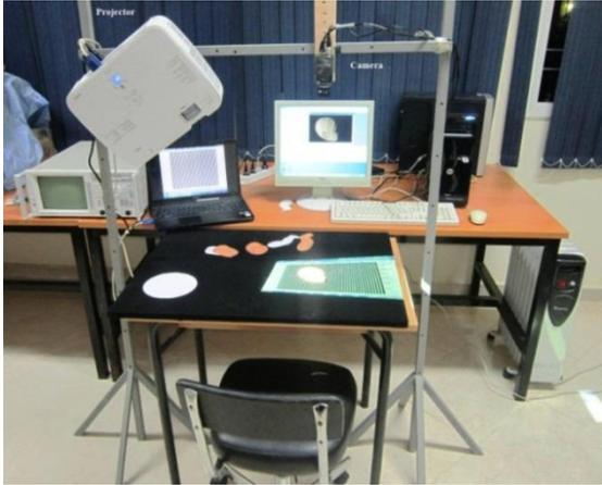
**Figure 7.** The fringe projection setup
