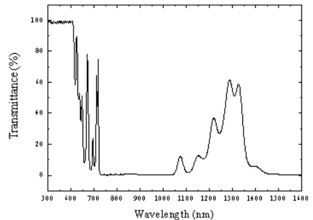
Figure 6. Mirror 2 of low transmittance to 976 nm and 1550 nm provided a 548 nm single wavelength output
