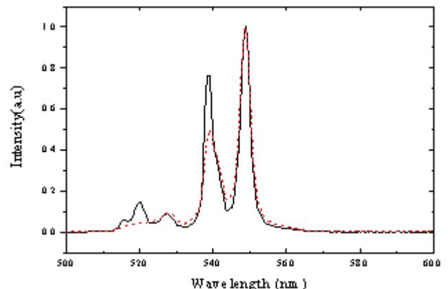
Figure 11. Fluorescence spectrum of the Erbium-Doped LiLuF<sub>4</sub> Crystal
