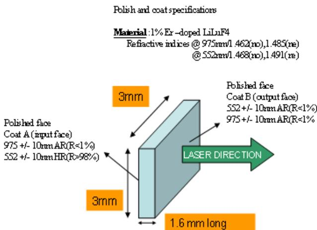
Figure 2. Polish and coating specifications of  $\text{LiLuF}_4$  crystal
