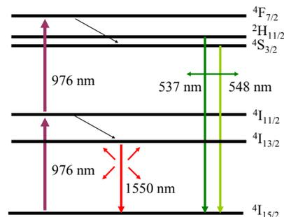
**Figure 1.** Energy level scheme of Er<sup>3+</sup>:LiLuF<sub>4</sub> with 976nm pump laser
