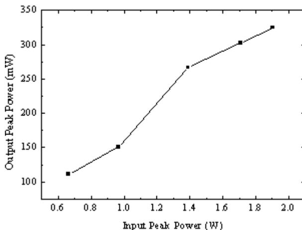
Figure 9. Input peak power at 1.9W can get max output power 320mW
