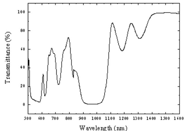
Figure 5. Mirror 1 appeared low transmittance to 548 nm laser and formed a 548 nm laser cavity with the coating on the face of  $\text{LiLuF}_4$  crystal
