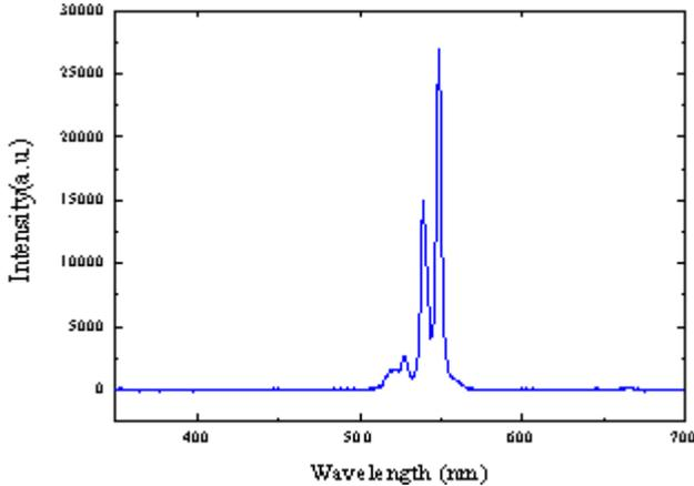
Figure 7. Maximum peak wavelength of output laser is 548 nm
