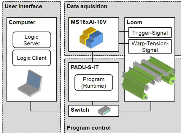
**Figure 17.** System architecture for implementation of control for fabric weight into the weaving machine
