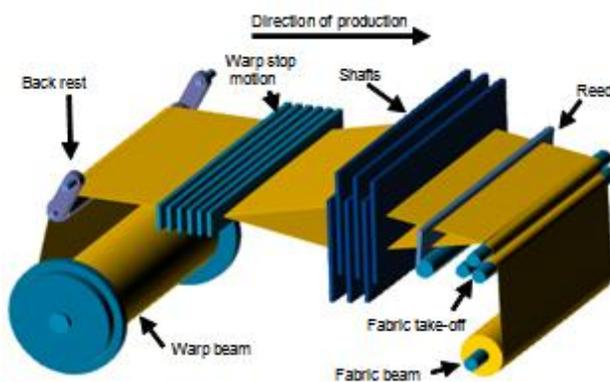
Figure 1. Principle of a weaving machine
