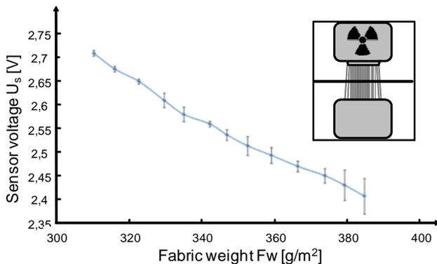
Figure 4. Correlation between sensor signal  $U_s$  and fabric weight  $F_w$
