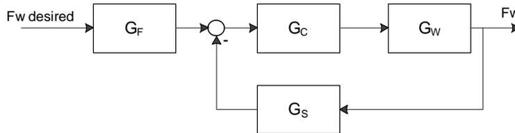
Figure 11. Simplified closed control loop
