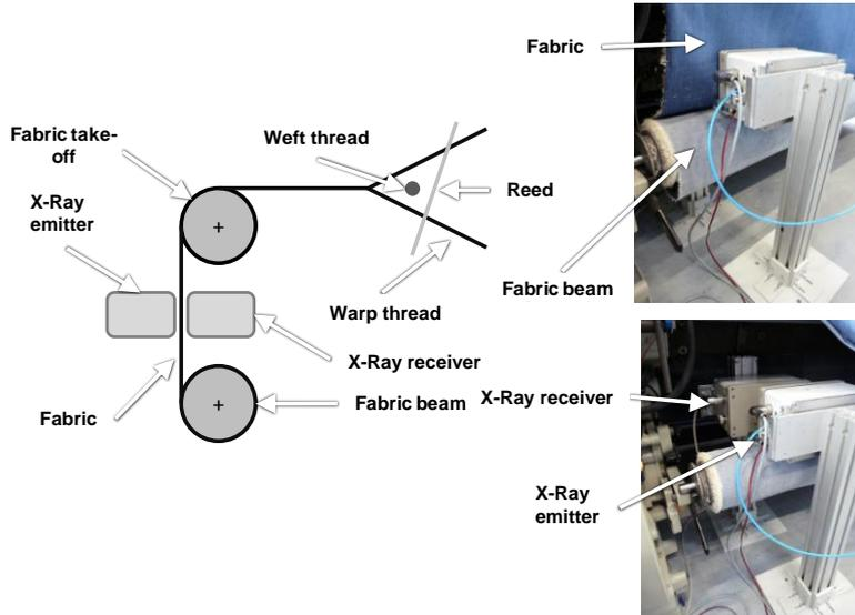
Figure 3. Installation of the X-ray system in the weaving machine
