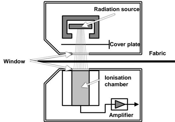
Figure 2. Principle of a X-Ray sensor system
