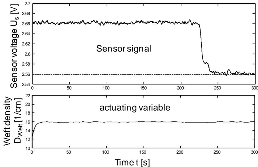
**Figure 18.** Behaviour of sensor voltage and weft density during control mode
