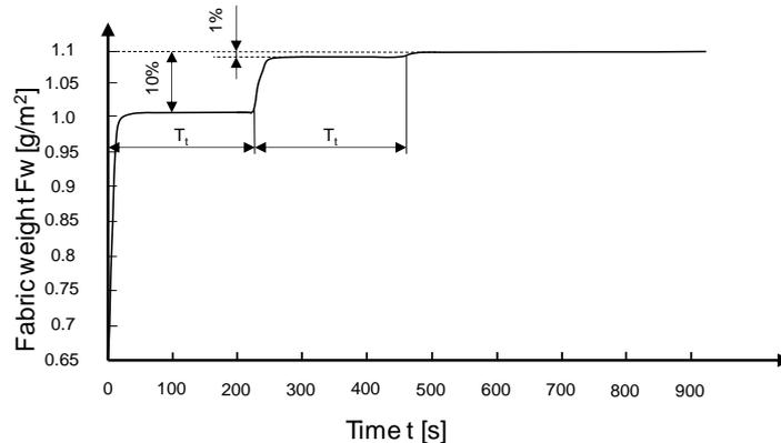
**Figure 15.** Step response of Smith predictor controller with defective transfer element of the sensor
