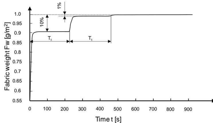
**Figure 14.** Step response of Smith predictor controller with defective transfer element of the weaving machine
