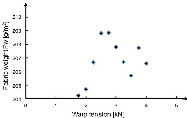
Figure 6. Correlation between warp tension and fabric weight Fw at constant speed and weft density  $D_{Weft}$
