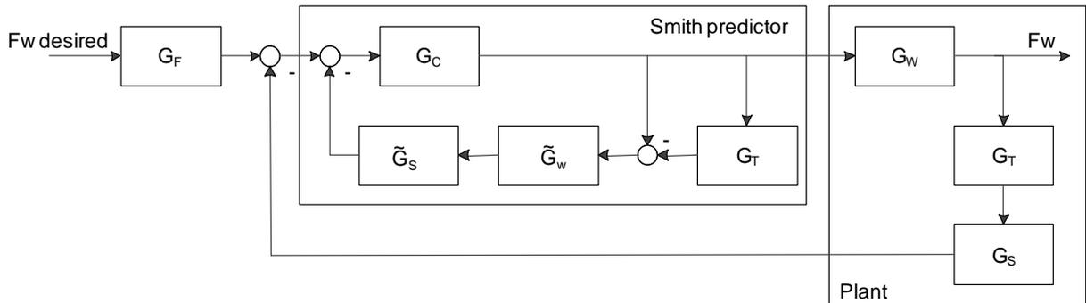
Figure 10. Closed control loop with Smith predictor
