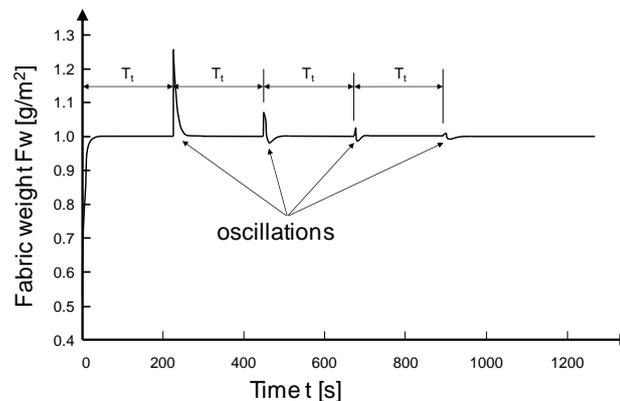
**Figure 16.** Step response of Smith predictor controller with defective transfer element of the dead time
