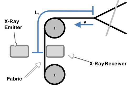
**Figure 8.** Dead time length  $L_t$  in the weaving process
