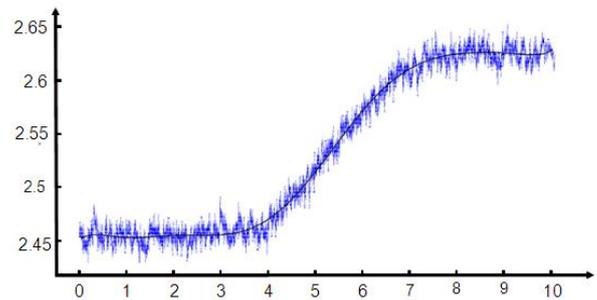
Figure 7. Step response of X-ray sensor
