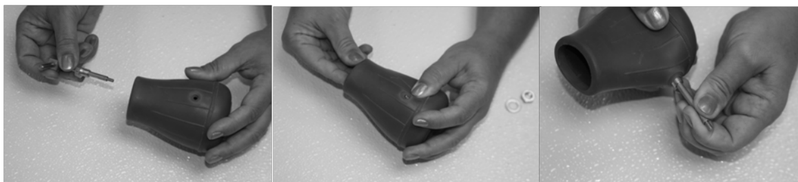
Figure 6. Insert the flint-type spark into the rubber bulb. Pull the spark out of the hole until the thread appears
