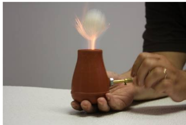
Figure 3. The combustion and expansion of the gas launches the ping pong ball
