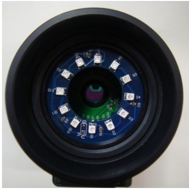
Figure 2. 375 nm LED ring-shaped light sources
