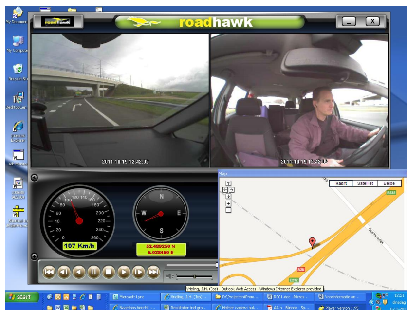
Figure 3. Screenshot of recording with Roadhawk RH2, upper left: a view of the road environment, upper right: a view of the driver, lower left: virtual dashboard with speed and heading, lower right: location on basis of GPS coordinates (Google Maps)
