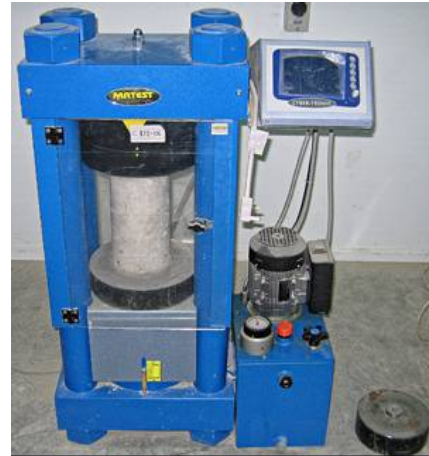
Figure 4. Compressive strength test of concrete
