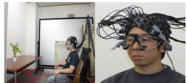
Figure 2. Experimental setting and physiological measures, eye marker and multi channel near infrared spectroscopy
