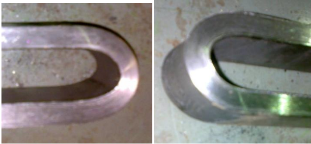
Figure 6. 2T Bend Tested Specimen
