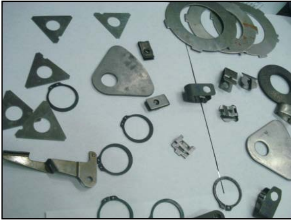
Figure 2. Items fabricated using MC 55 grade steel
