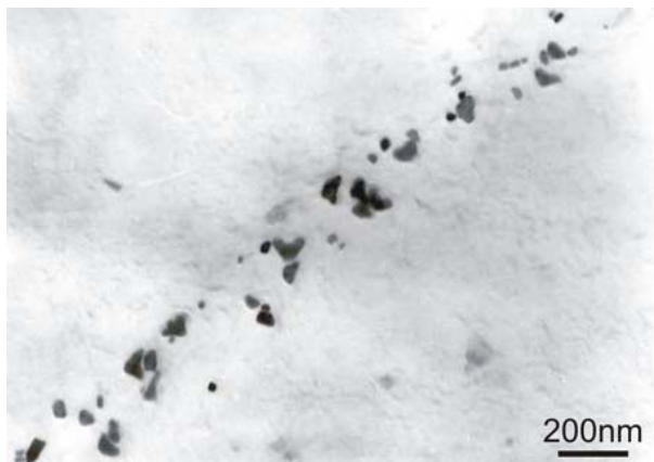
Figure 6. TEM micrographs showing cruciform particles in a V-Ti-N steel (left), and cuboid particles in a V-Nb-Ti steel (right) after equalization at 1100°C.[8]
