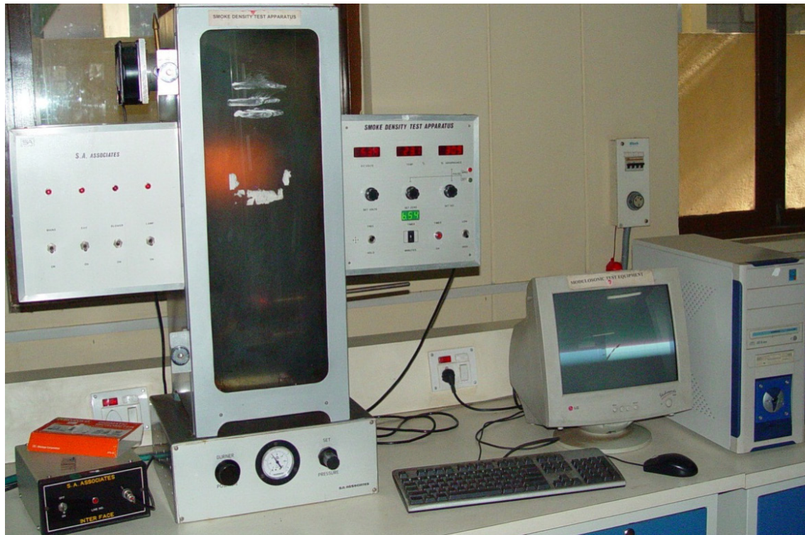
Figure 1. Computer interfaced Smoke density equipment
