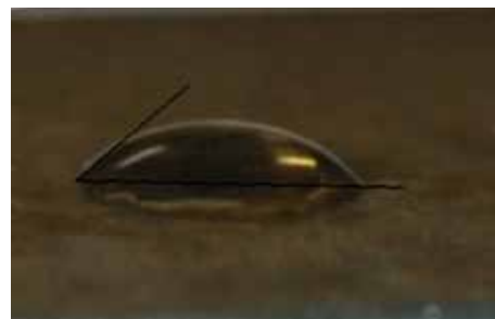
Figure 9. A water contact angle measurement on CdS:CuS composite thin film surface
