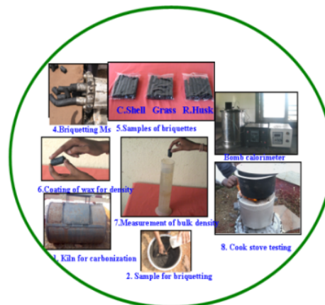
Figure 12. Complete setup for briquettes preparation and testing
