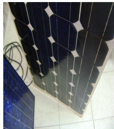
Figure 4. Monocrystalline solar cells interconnected and encapsulated within a solar panel
