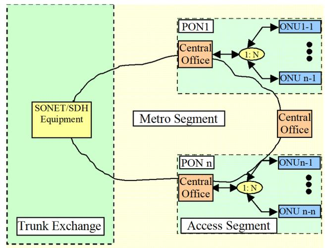
Figure 1(a). Basic telecommunication network
