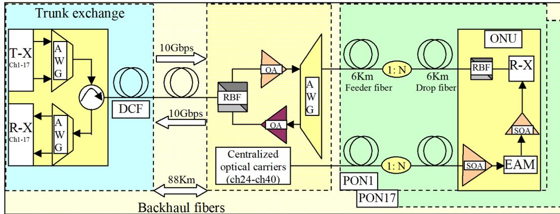
Figure 5. The centralized optical carrier TDM/DWDM-LR-OAN
