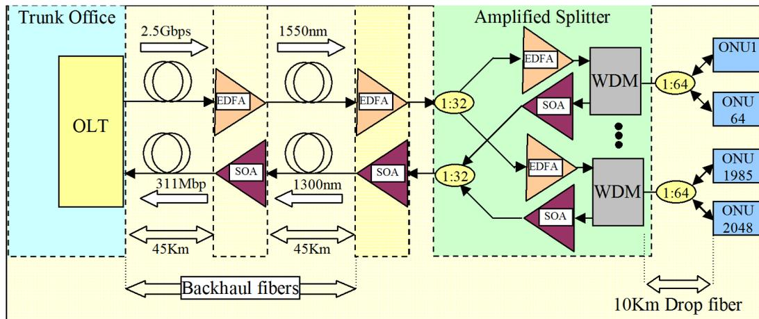
**Figure 2.** The SuperPON architecture
