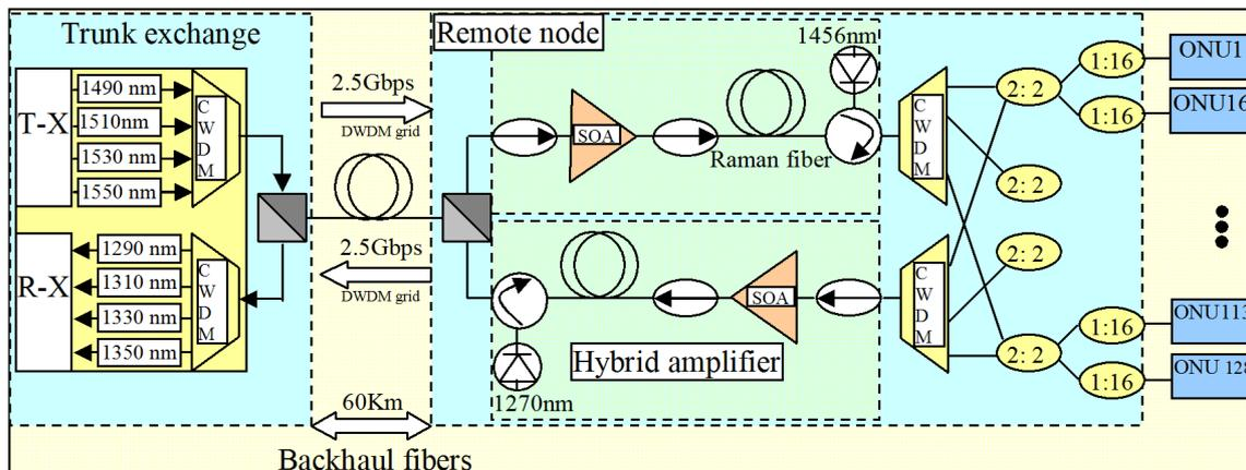
Figure 4. TDM/CWDM-based LR-OAN architecture
