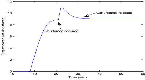
Figure 2. Set point and disturbance response
