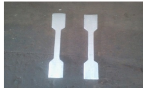
Plate 5. Prepared Sample for Tensile Test
