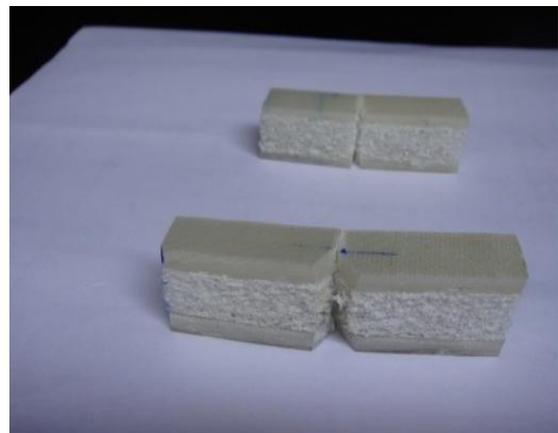
**Figure 4.** Fractured specimen under Izod impact test
