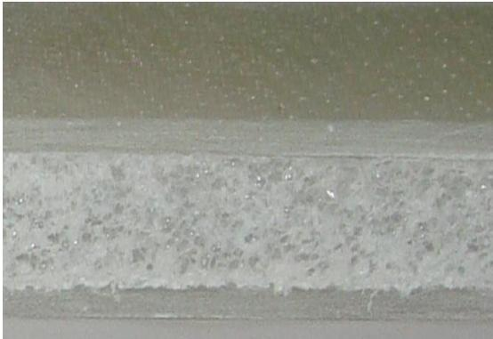
**Figure 1.** Sandwich structure of GFRP - polyurethane foam-GFRP
