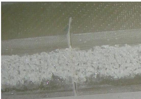
**Figure 2.** Notched GFRP-foam-GFRP composite
