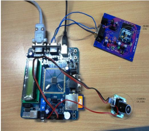
Figure 3. Sensor Node with Camera for image acquisition
