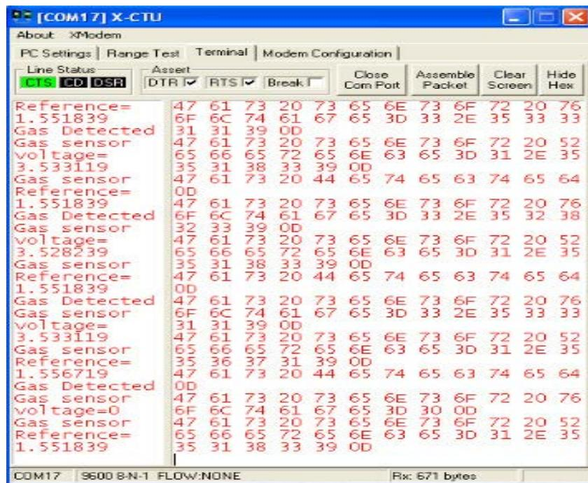
Figure 9. Data transferred from Gas sensor to base station
