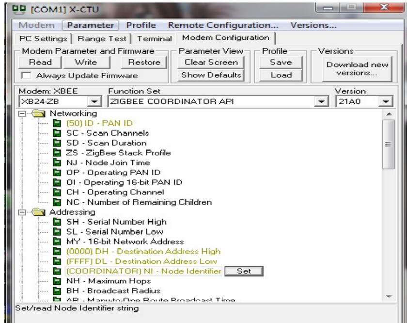
Figure 8. Configuration of xbee radio
