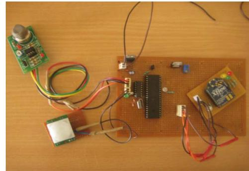
**Figure 2.** Sensor node for redetection of Intruder and Gas leakage
