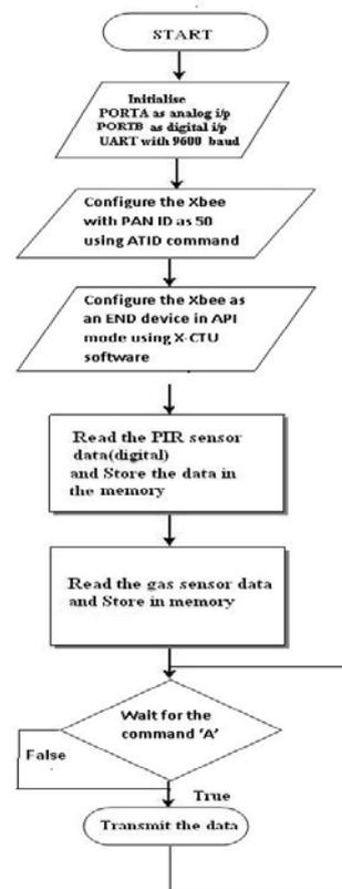
Figure 5. PIR and Gas sensor flow chart
